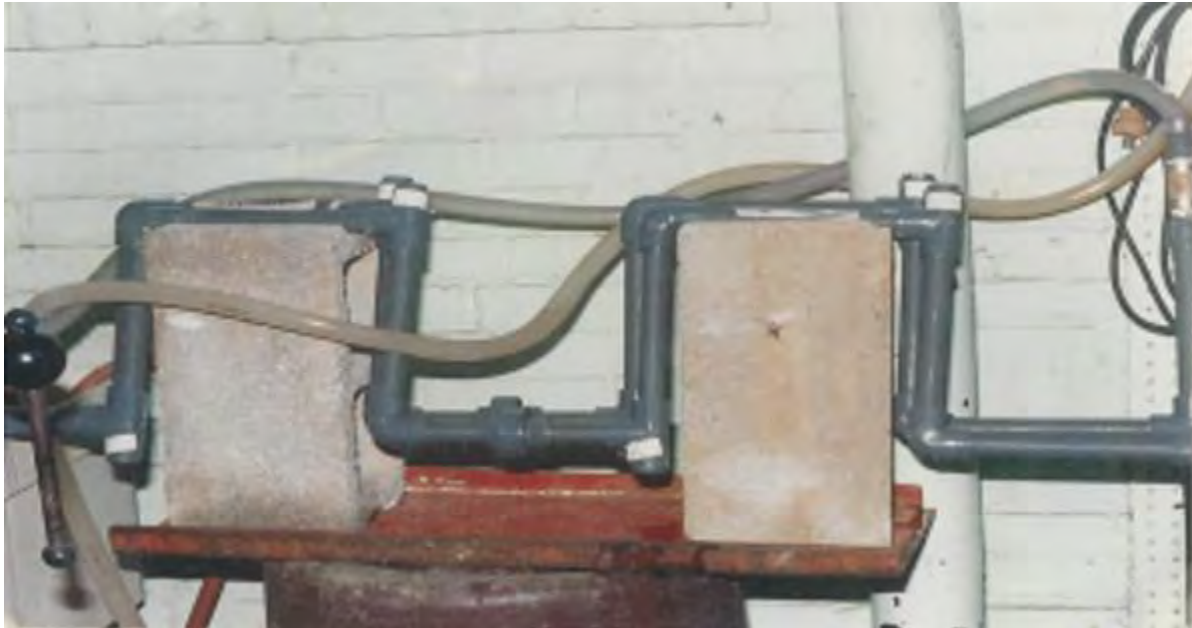
Image 2: Atlanta Coupon Loop Testing Apparatus
