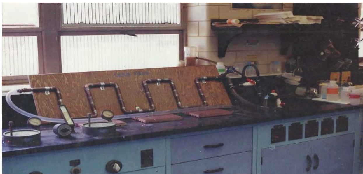
Image 1: Atlanta Pipe Loop Testing Apparatus
